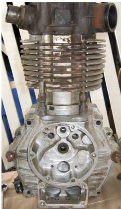
The 'Type 6' JAP, with beefed up crankshaft and main bearings, and an Alfin barrel on an aluminium crankcase, was designed for 500 racing. This one found its way to Rockhampton, Qld. Photos: Paul Stanley.
