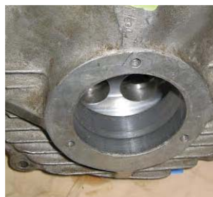
The 'Type 6' JAP, with beefed up crankshaft and main bearings, and an Alfin barrel on an aluminium crankcase, was designed for 500 racing. This one found its way to Rockhampton, Qld. Photos: Paul Stanley.
