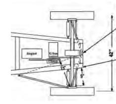
If radius arm pivot point went to here then radius would be about 15" which is much better than any conventional wishbone arrangement
